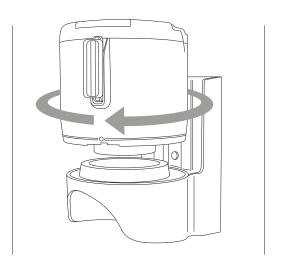
Ensure the Belt Barrier is located and locked correctly into its designed holder.
