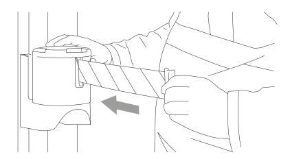
When releasing the retractable tape from the receiver, always walk the tape back to the fixed housing unit. Letting go of the tape from any distance could cause damage to the unit and inflict injury to anything or anyone in its path on its route back to the fixed unit.
