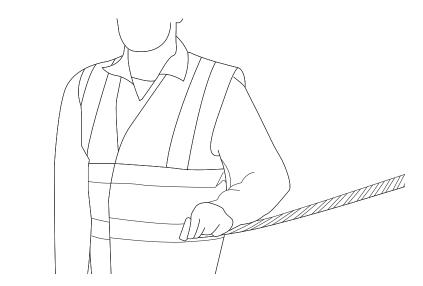
Pull the retractable tape from the unit to the desired length.
