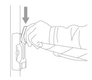
Locate the retractable tape end into the receiver plate ensuring it is pushed to the bottom of the unit.
