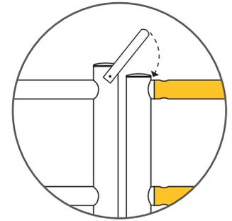
Gate Hasp option is recommended for both post to post and gate to post options.
