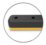
The twin layered Monoplex product offers a softer upper layer which dissipates energy whilst the lower harder layer provides rigidity around the fixing holes. This ensures the Step Guard remains strong under impact and distributes energy across the product, reducing the risk of damage and minimizes the risk of fixings pulling out of the ground.
