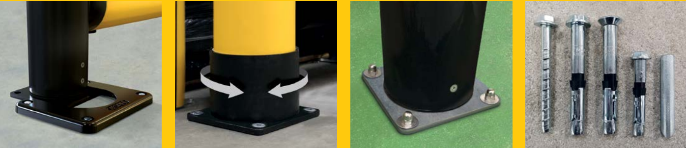
Slider plates to allow guardrails to be removed for easy access. Spinning collars to increase deflection of glancing blows. Multiple base plate options: galvanised, stainless steel and countersunk. Anchor bolt varieties to suit different floor substrates.
