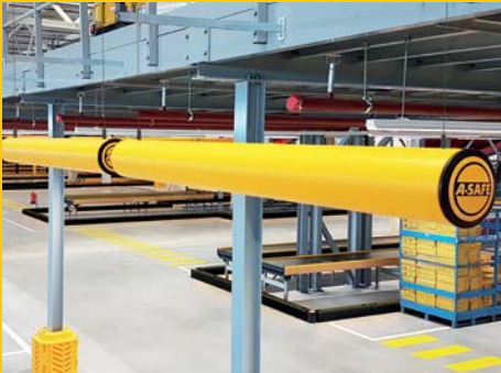
Multiple Alarm Bar safeguarding an overhead structure.
